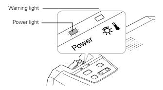
If the projector is not working correctly, first turn it off and unplug it. Then plug the power cord back in and turn on the projector. If this does not solve the problem, check the status lights on top of the projector and try the solutions recommended below.
