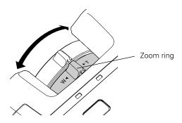
You can also change the image size by moving the projector closer to or farther away from the screen. You can use the **E-Zoom** buttons on the remote control to zoom in on a portion of the image. See page 33 for instructions.
