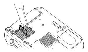
If the dirt is difficult to remove or if the filter is torn, replace it. Contact your dealer or call EPSON at (800) 873-7766 to obtain a new one. In Canada, please call (800) 463-7766 to locate a dealer.
