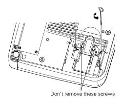
6. Hold the lamp by the top, as shown, and pull the lamp straight out.
