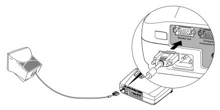
3. Connect one end of the computer cable to the projector's Computer/Component Video port, as shown.
