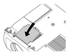
7. Replace the filter cover by inserting the tabs and then pressing down the other end until it clicks into place.
