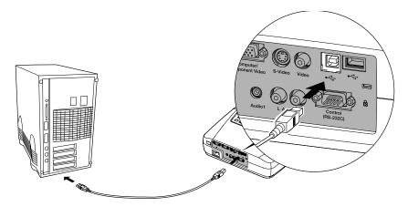
2. Disconnect your Macintosh's mouse cable. Connect the other end of the projector's mouse cable to a USB port on your Macintosh.
