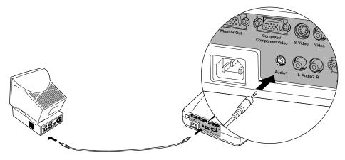
2. Connect the other end of the audio cable to the speaker or audio out port on the computer's sound card.
