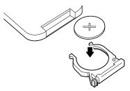
3. Slide the battery tray back into the remote until it clicks into place.
